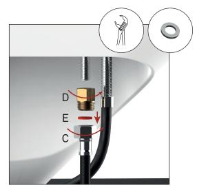
2.2 - Pass the hose (C) through the hole of the vacuum breaker.
