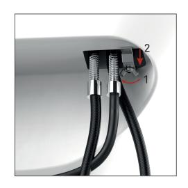
1.2 - Remove your regular showerhead from the vacuum breaker by pulling it out of the hole
