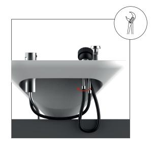
Note: If it's too difficult to access the hose to unscrew it, you can disassemble the vacuum breaker from the backwash. To do that, unscrew the wing nut (1) of the vacuum breaker and remove it from the holding bar (2). You can then pull out the holding bar. You can then loosen the vacuum breaker from the hole in the backwash.
